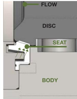
The pressure is transferred to the underneath of lip edge when the pressure comes to the pressing ring side, and this can further increase the sealing force between disc and seat.
