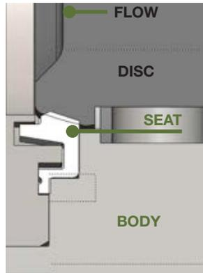
The disc is pushed to the seat as the pressure applied to the non-pressure side of the ring. And it will be more and more tightly closed as the disc is close to the spherical seat. The contact between the lip edge and bottom groove of pressing ring can limit excessive movement of the seat.
