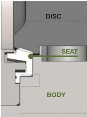
The seat is slightly deformed as the valve closed. And this deformation inspired seat to maintain a lasting sealing with the edges of disc.
